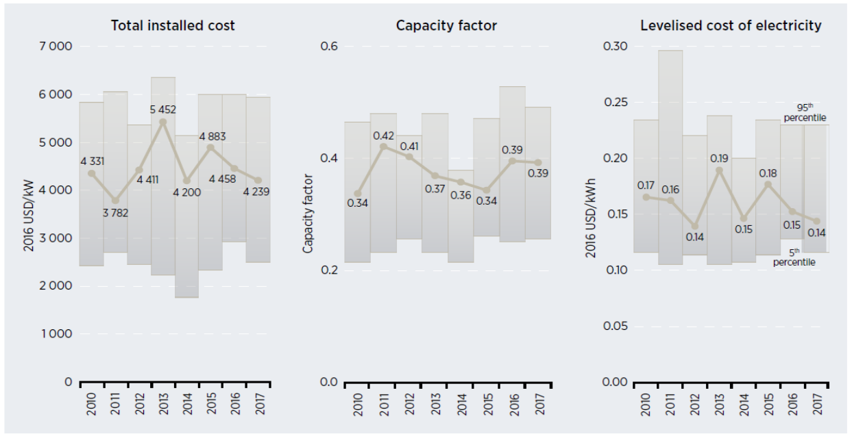
Global weighted average total installed costs, capacity factors and LCOE for offshore wind, 2010-2017
